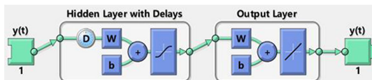
Fig. 1 The configuration of the NARNN. The NARNN consists of one output layer with 1 unit and one hidden layer with n units and D delays
